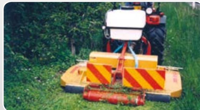
The **herbicide spraying system XID** may be mounted to many SEPPi mowers. High-precision nozzles come with adjustable spraying direction.
