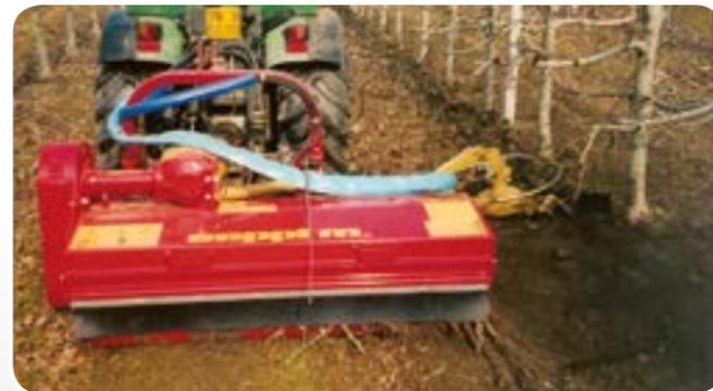
With the **sweeper XAN** you may collect leaves and prunings from row sides and bring them into an ideal position for mulching: in front of the mulching mower.
