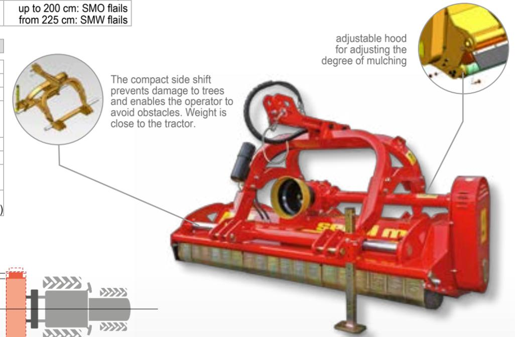
The compact side shift prevents damage to trees and enables the operator to avoid obstacles. Weight is close to the tractor.
