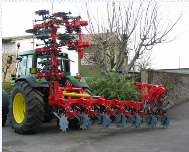
INTER-ROW CULTIVATOR WITH HYDRAULIC FOLDING FRAME
