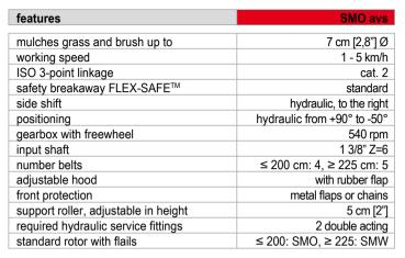
**SMO** avs is a very strong offsetting mower. It mulches grass and brush up to 7 cm [2.8"] in diameter. Hydraulic angling and hydraulic side shift make it possible to work in many different positions and situations. It is suitable for the maintenance of greenspace such as slopes, road sides, or of steep orchards and vineyards. As on all the SEPPI flail mowers, it is possible to adjust the height of cut and the degree of mulching.
