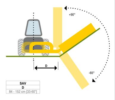
The offsetting mulcher SAV comes with hydraulic angling from  $90\ensuremath{^\circ}$  up, to  $65\ensuremath{^\circ}$  down.
